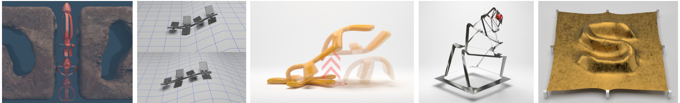
Fig. 1. Our computational framework, supporting both forward simulation and inverse design of magnetoelastic thin shell structure, can realize various applications, ranging from forward locomotion generation, quasi-static shape design, to motion planning. From left to right, the images present: a swimming octopus, a crawling reptile robot, a jumping starfish, a deforming Kirigami tower, and an embossed letter.
