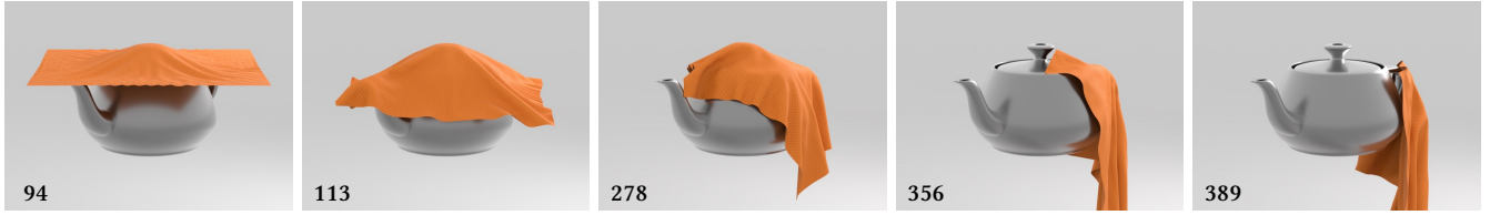
Fig. 7. A square sheet of square cloth ( 20 \times 20 bicubic Hermite patches) drapes on a teapot (32 bicubic Hermite patches) under gravity, eventually sliding down along the handle. The simulation runs smoothly and stably at a 2 ms time step, with no visible interpenetration between cloth and teapot.
